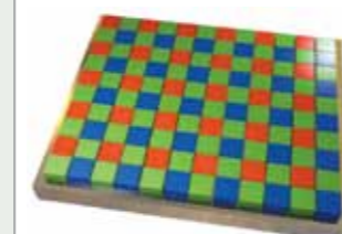
▲ A Bayer filter mosaic contains twice as many green photo sensors as it does red or blue. Some arrays have a different configuration to this example but the end result is always the same
